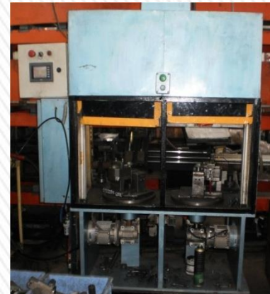
Twin stage rotary welding machine w/ fixture
